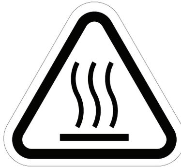
**Fig.1.6 (b) High-temperature warning label**
